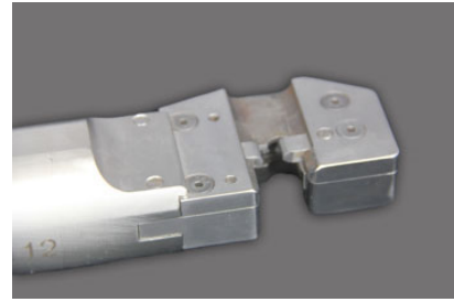
C-style handset with parallel action jaw set. Teamed with hydraulic pump (not shown). Custom build-to-order tool.
